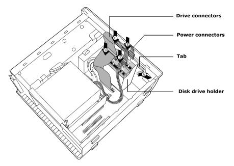
10 Push in on the tab (A) to securely latch the holder to the chassis.
